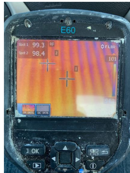
Temperature on Top of Super Therm® 98.4 Degrees F
